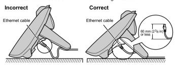
Use a straight CAT 5e (or higher) Ethernet cable (not included) that is 6.5 mm (<sup>1</sup>/<sub>4</sub> in) in diameter or less.
